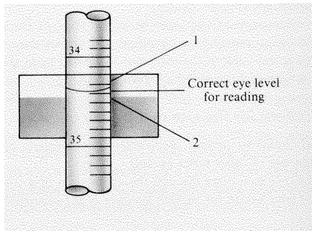
read a buret with a repeatable precision of  $\pm 0.01$  mL so as to eliminate this source of errors in all of the volumetric analyses that you perform. What is the volume of the liquid in the buret shown above? Does that volume agree to within 0.01 mL of the volume proposed by your instructor?
